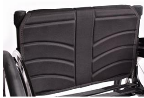
EXO superlight (KRF030005): lightweight version of the EXO backrest upholstery. EVA-foam padding, adjustable straps, wider cut of the upholstery to cover backrest tubes (-160 g compared to Std. EXO backrest-upholstery)
